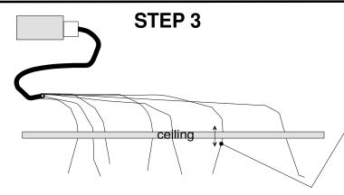
Apply a small amount of <u>epoxy glue</u> at this point, work the fibre up and down so as to line the hole in the ceiling with glue and not have any below ceiling level.
